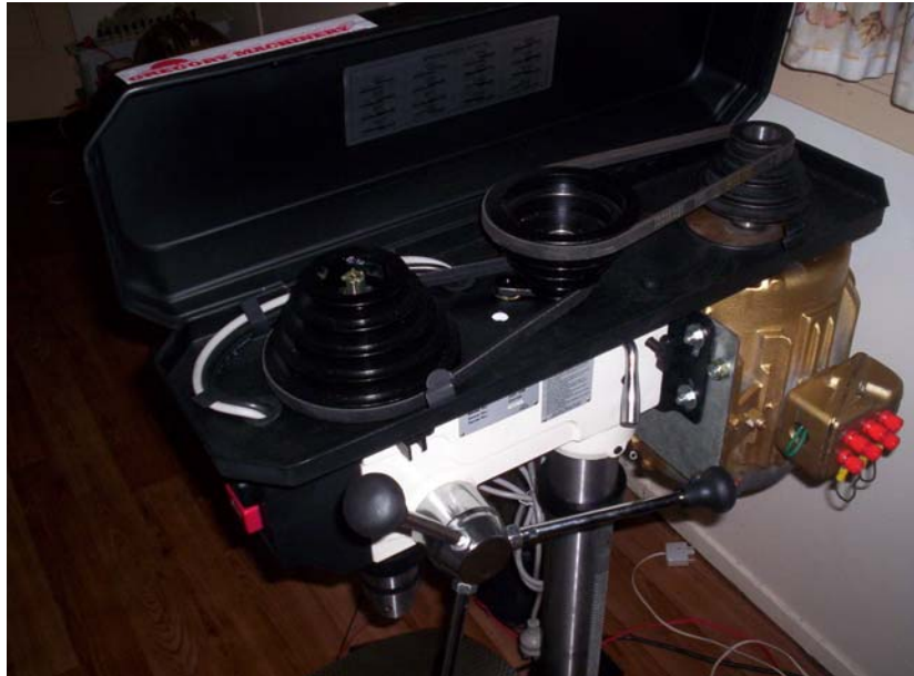
Example of a modified Floor Drill press with an RV motor
